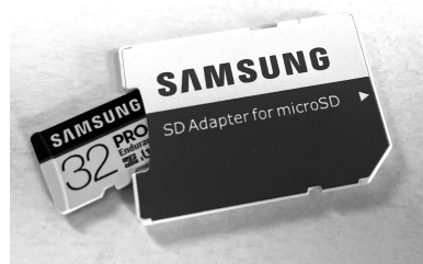
Figure 1.3: microSD card and SD adapter.
