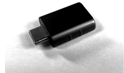
Figure 1.6: USB-C to USB-A adapter.
