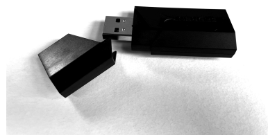
Figure 1.4: USB-to-SD card reader/writer.
